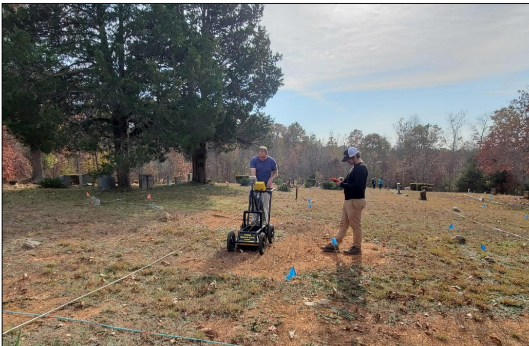
Figure #13: GPR Survey in progress, Union Baptist Church (Shores) Cemetery.
